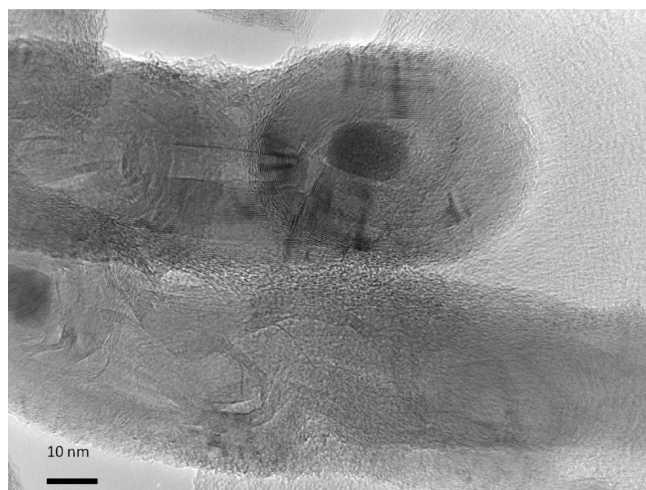
Figure 12. TEM image of a catalytic nanoparticle enclosed in the nanotube.
